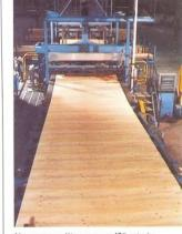
Veneer travelling at over 150 m/min. through Rotary Clipper.
