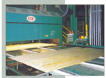
Several man years in development, Coe presents the Veneer/Lumber Grade Scanner for automatic sorting and stacking. It inexhaustibly monitors your sorting line and makes accurate grading decisions piece by piece.
