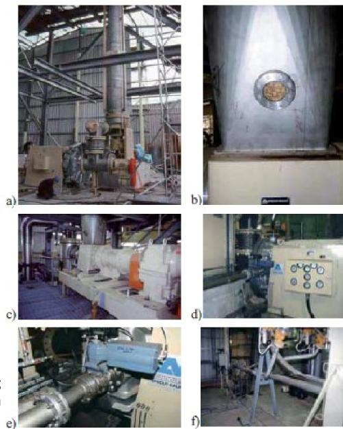
a- tube; b- window; c- pluging screw; d- main engine; e- blow pipe; f- resin injection
